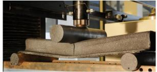
Figure 5: 3-point Flexure Test Setup
