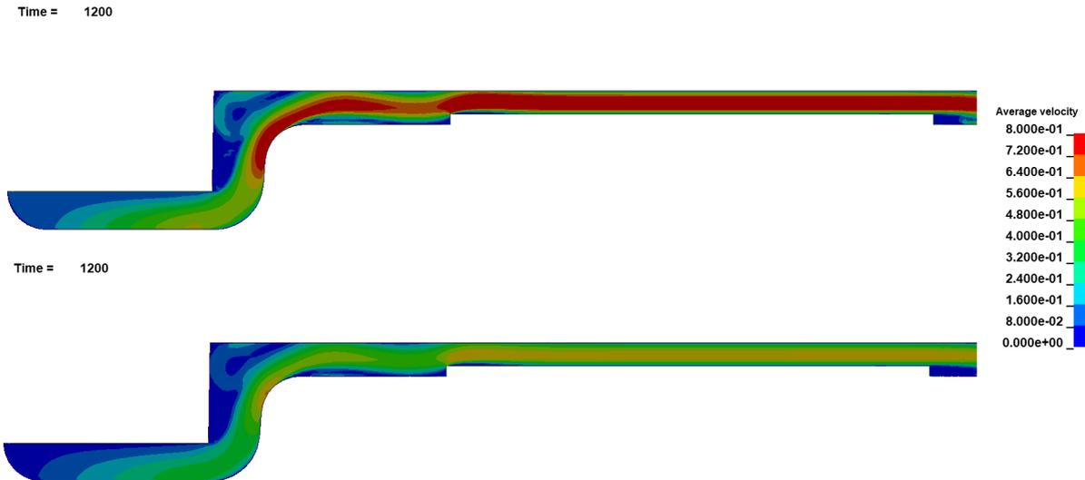
Fig.7: Average velocity for tests 2 (top) and 3 (bottom) after 1200ms
