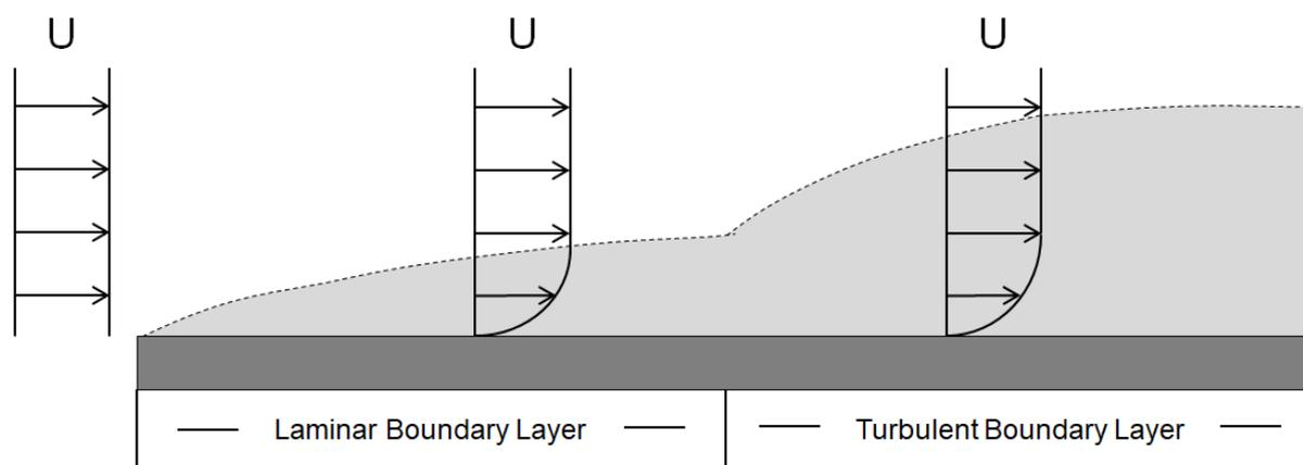
Fig. 1: Typical flow regime found on a flat plate
