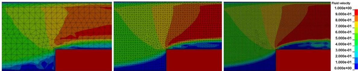
Fig.4: Velocity Contours for Grid Refinement Levels 1, 4 and 9.
