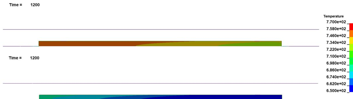
Fig.6: Insert Temperature for tests 2 (top) and 3 (bottom) after 1200ms
