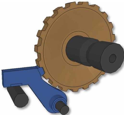
For the gearbox park brake system a topology optimisation was performed to determine the optimal material distribution for the locking arm and main gear, considering both clockwise and counter-clockwise torque loadings of the transmission. The optimisation therefore considered two implicit LS-DYNA models during the study.
