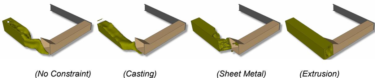
Figure 8: Pole Impact Topology Results for Different Manufacturing Constraints
