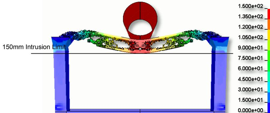
Figure 7: Maximum Dynamic Intrusion of Topology Pole Impact Result
