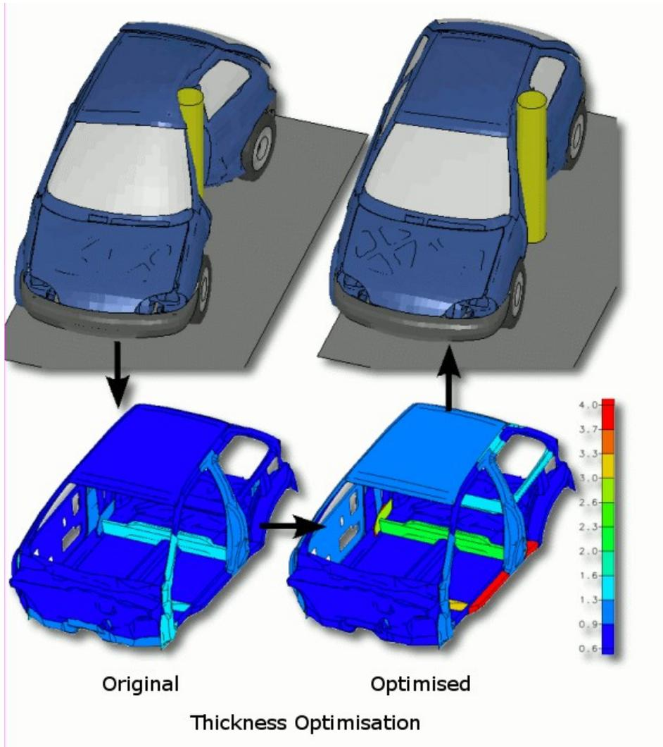
Figure 9: Sizing Optimisation Results of Vehicle Pole Impact & Body Torsion
