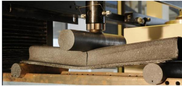
Figure 5: 3-point Flexure Test Setup
