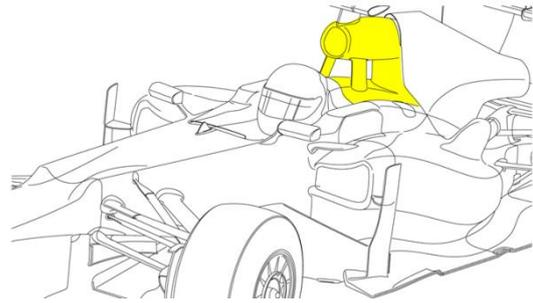
The Load Case/ Assumptions provide a rear loading primary load case for optimisation and use LS-DYNA coupled with Genesis to simulate it, loading forward simulation as the linear load case in Genesis.
