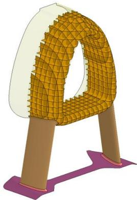
For this particular project the maximum displacement of 20mm is considered for a primary loading, given a test limit of 25mm, with no structural failure allowed 100mm below the top of the roll hoop. This is achieved through stress and composite failure limits.
